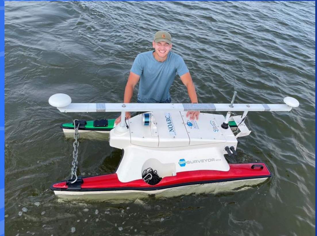
Sea Robotics Surveyor Autonomous Surface Vehicle equipped with an EdgeTech multibeam sonar.
