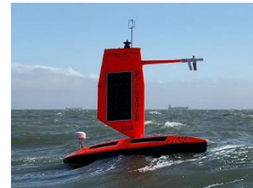
3: Obtain critical surface level observations in storm center using Sairdrone USV
